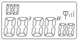
2. Press<CLR> for more than 2 seconds, the memory will be cleared, and signal receiver will be turned on; The LCD will show:
